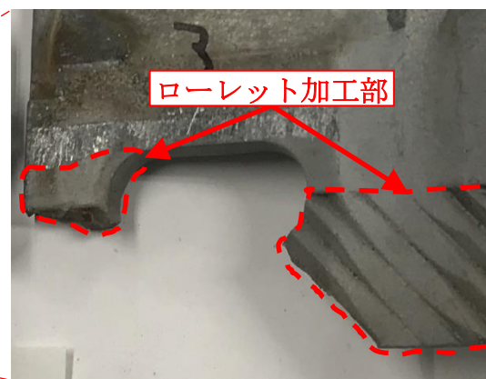
(c) 孔縁端部の破断 (支柱④)
