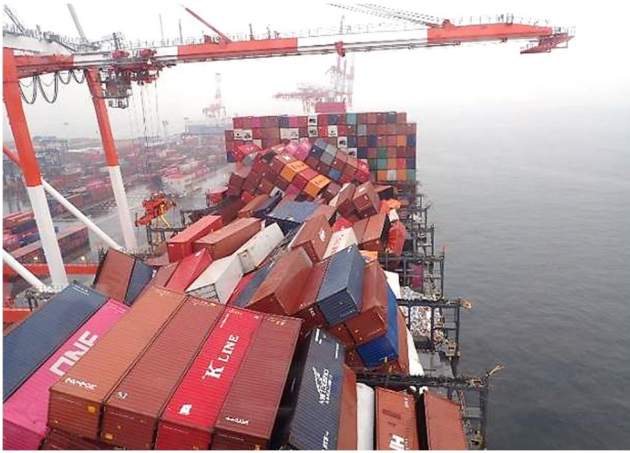
Photo 6 Collapsed containers on upper deck
