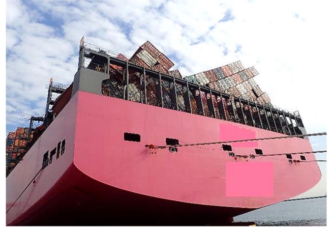
Photo 9 Collapsed containers at stern
