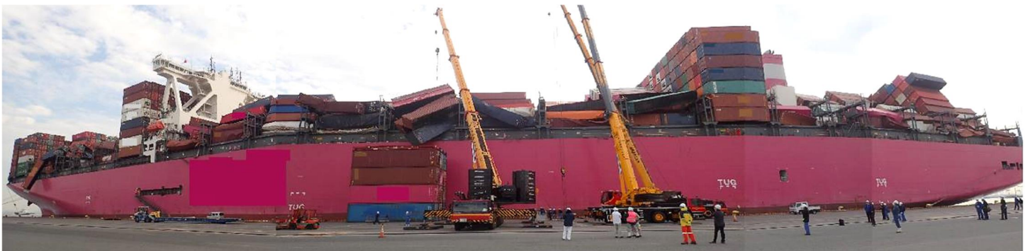
Photo 5 The collapsed container seen from the port side
