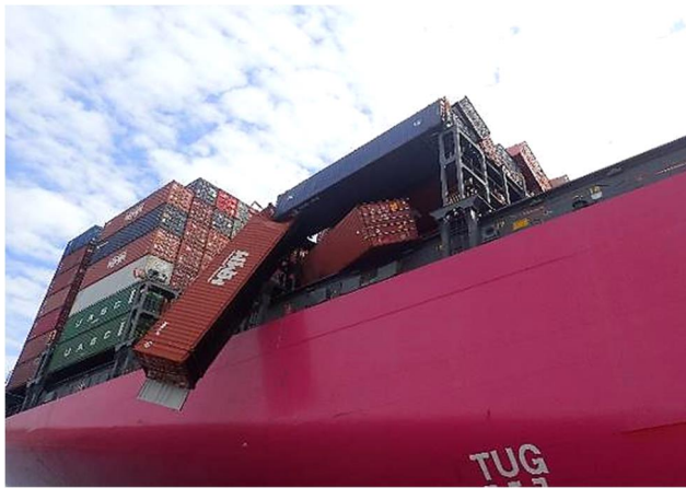
Photo 8 Containers on the verge of falling
