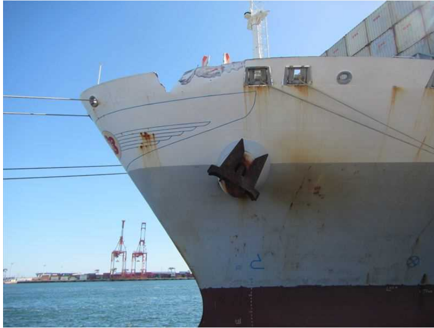
Figure 5 State of damage to the Vessel (Bulwark on the port fore part)
