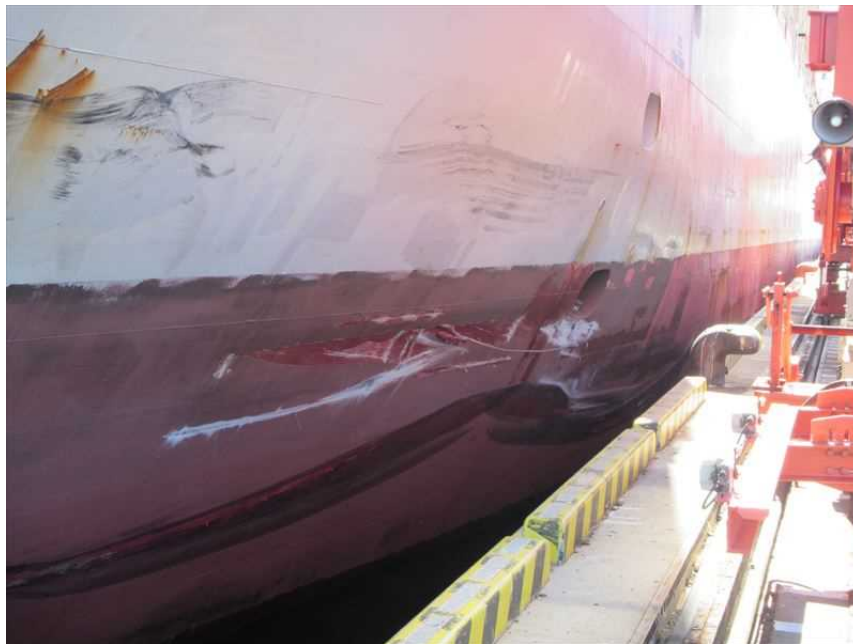
Figure 6 State of damage to the Vessel (Port fore part shell plate)
