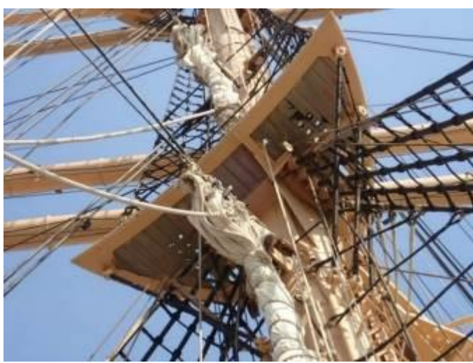
Picture 2.5-2 Rope going through a top board
