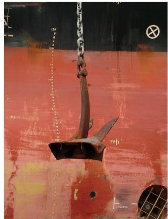
Damaged recessed port anchor shank
