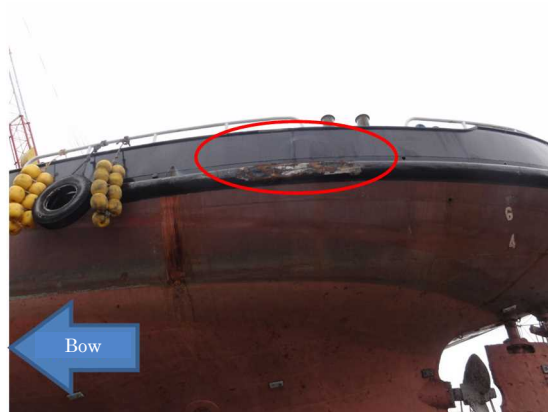
Photo 2.3-4 Damage to the port stern (Vessel B)
