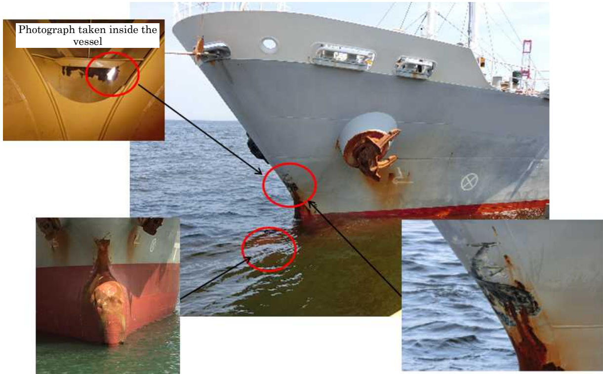
Photo 2.3-1 Damage to the bow (Vessel A)
