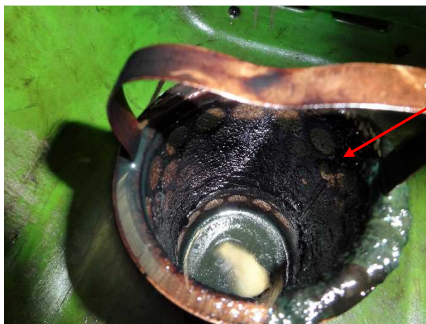
Photo 2.9-2 Clogging condition of strainer①
