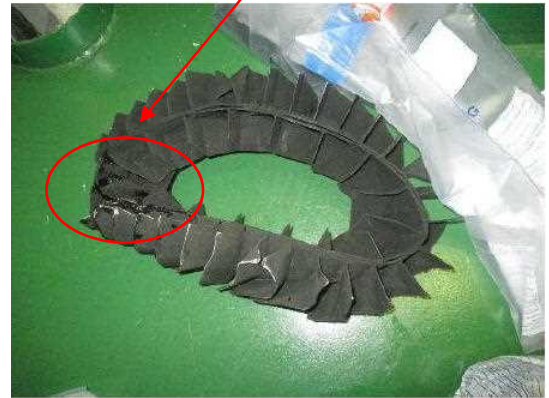
Photo 2.3-2 Secondary air nozzle damage condition
