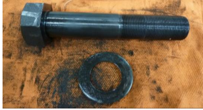
Photograph 2: Same type of bolt as the hold-down bolt
