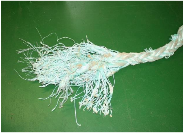
Photo 2-3 Severed End of the Line
