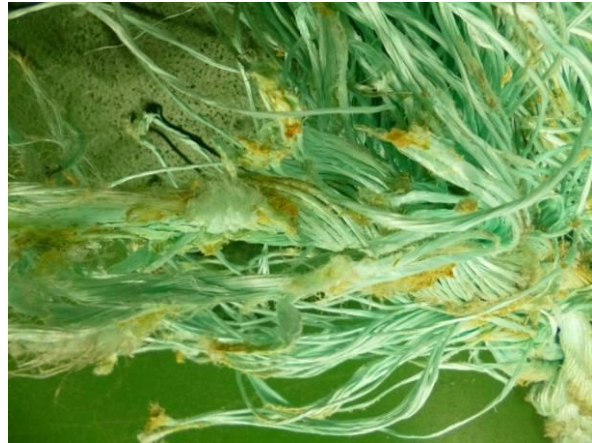
Photo 2-4 Melt Marks on the Severed End of the Line
