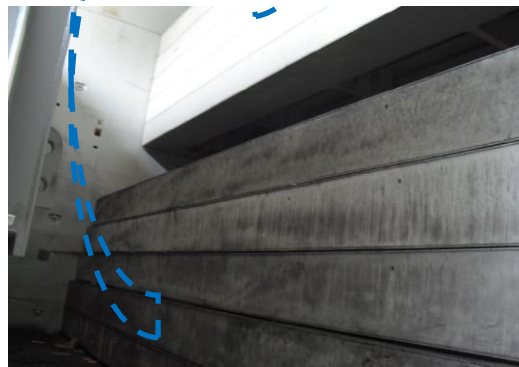
Photo 2.1-6 Tween deck hatch covers that were placed on the bow side of the inner bottom plating in No.2 cargo hold (Photographed during a previous voyage, prior to the accident)
