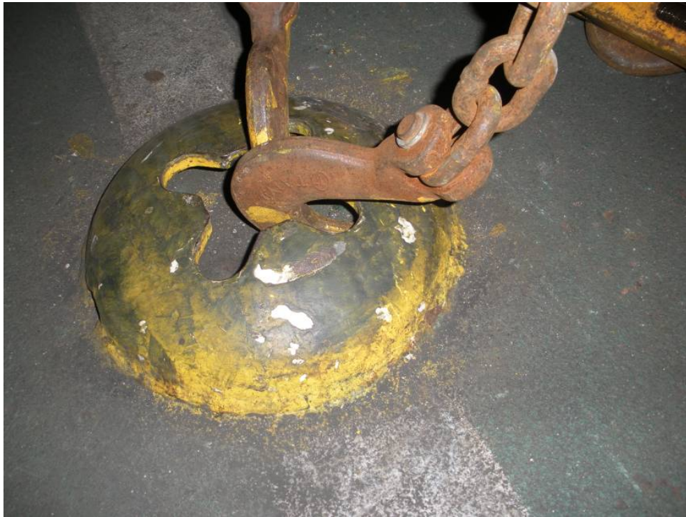
Photo 7: Lashing Chains Hooked on Cloverleaf
