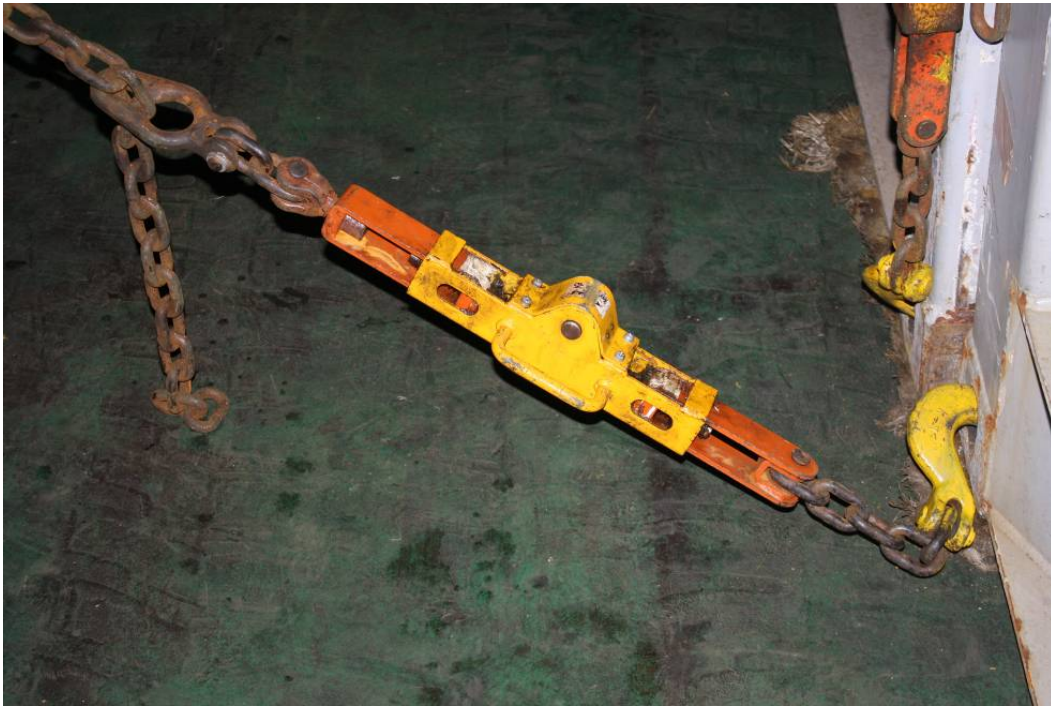
Photo 9: Twisted Hook of Lashing Chain
