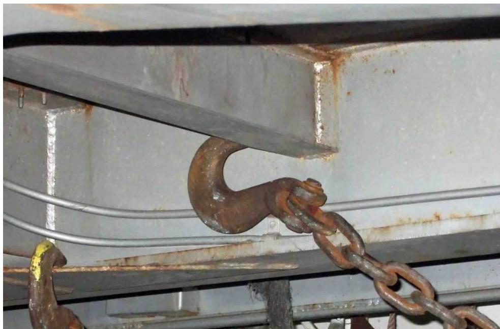
Photo 8: Lashing Chain Hooked on Member at the Back of Chassis's Body
