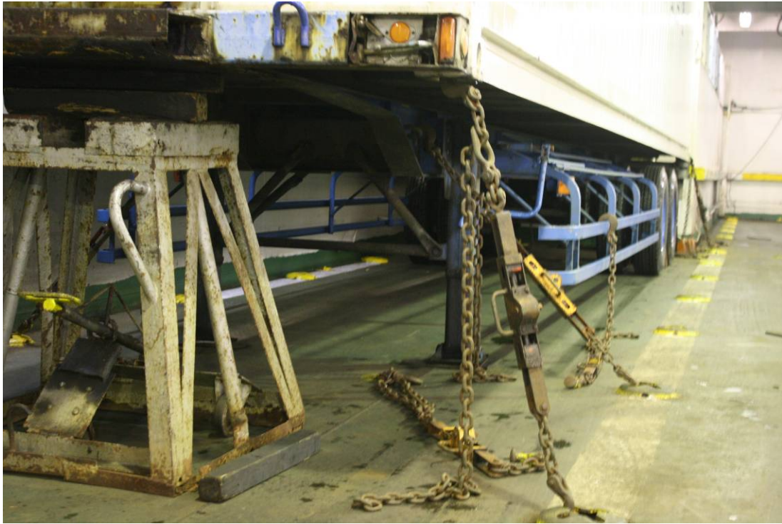
Photo 5: Lashing Condition of Chassis (6- Point Lashing Chain)
