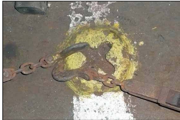
Point of contact (45°) between a hook and a cloverleaf (projecting type)
