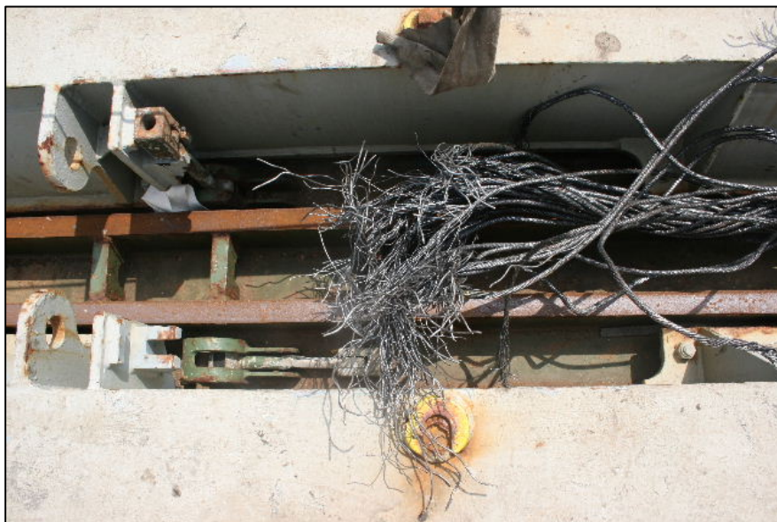
Picture 6—the Main Wire at its Break Point
