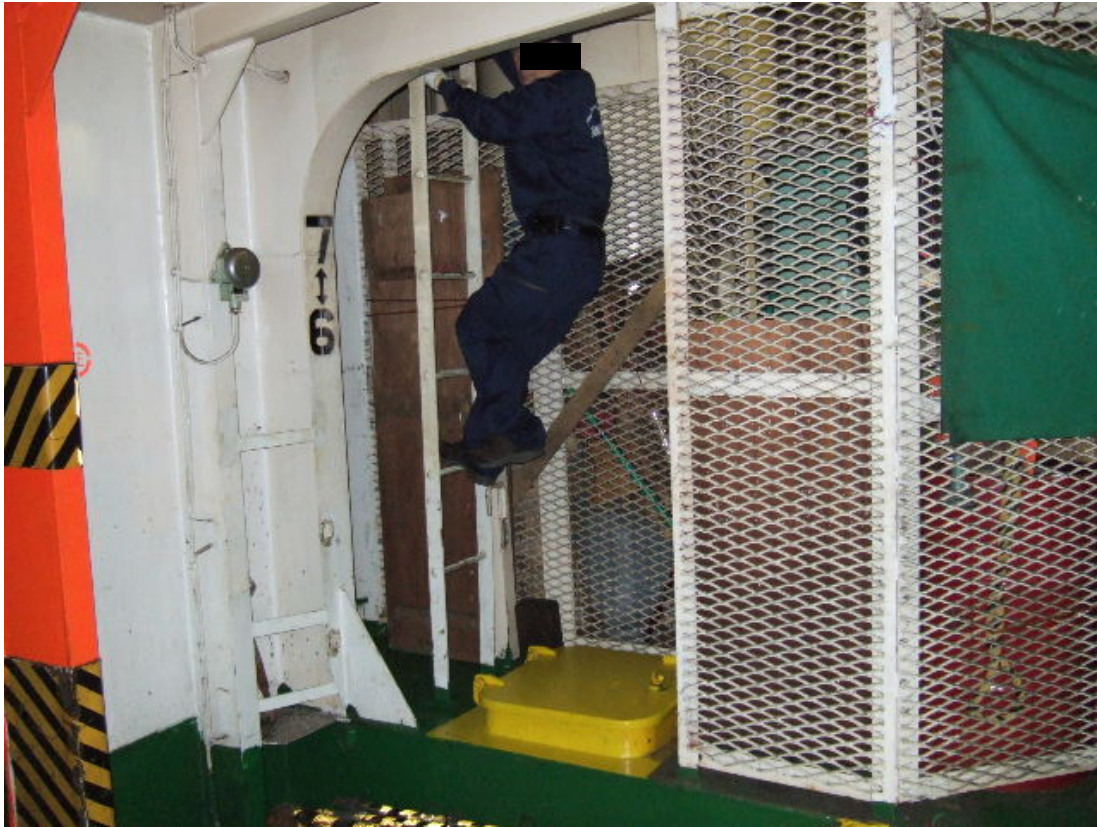
Photo 5: Vertical Ladder Connecting DK 6 and DK 7
