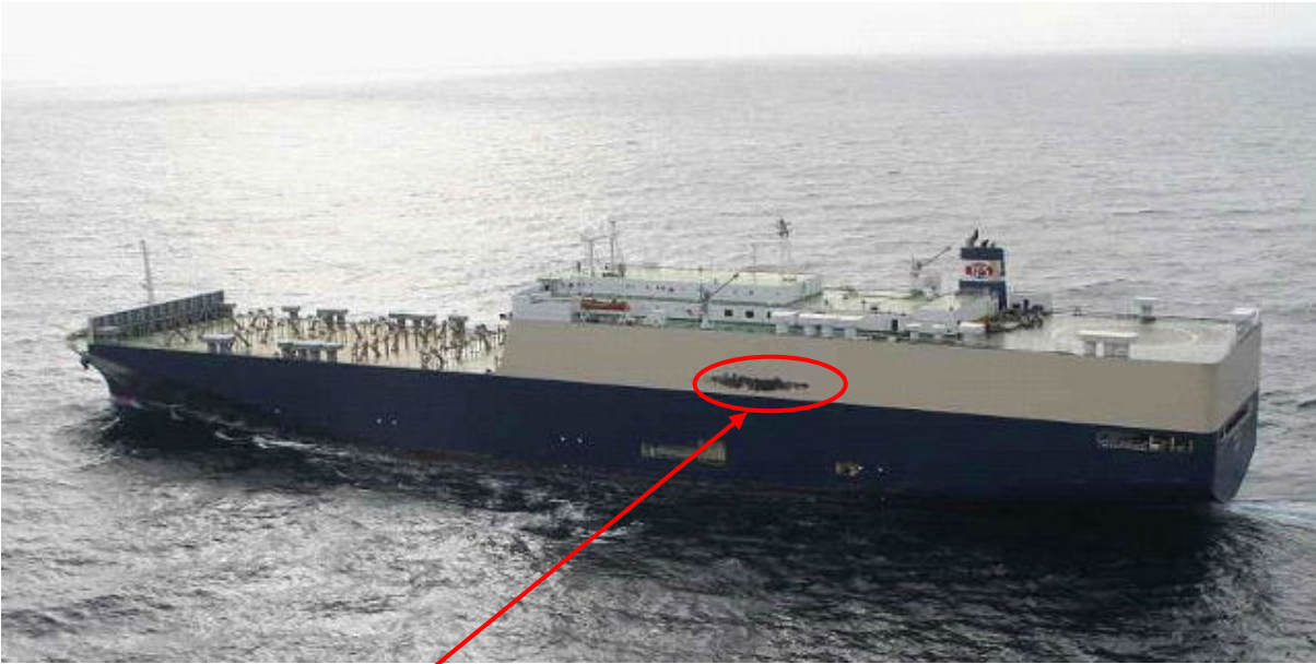
Paint was burnt away
