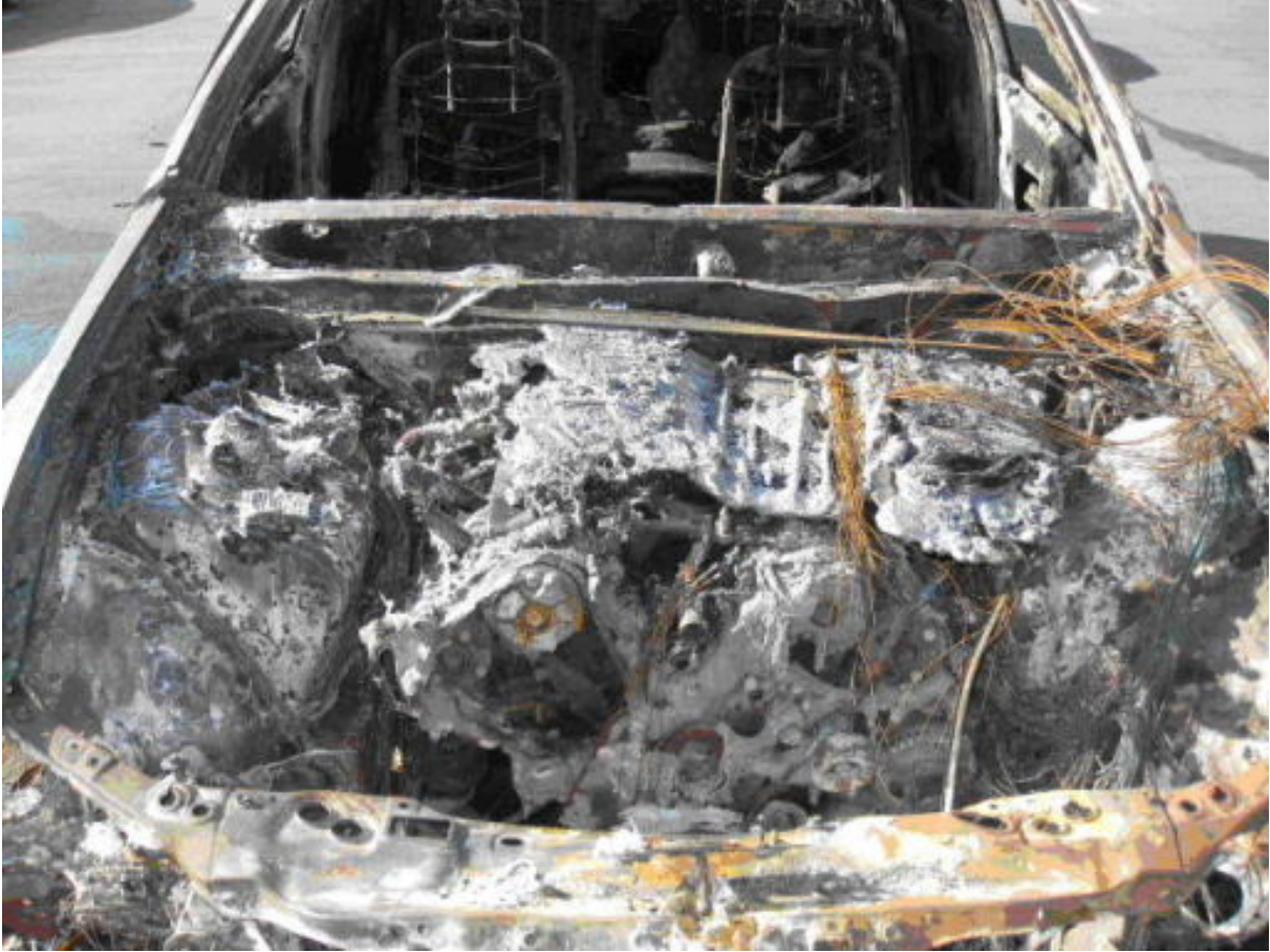
Photo 16: Fire Damage Situations of Car 10-07 Engine Bay
