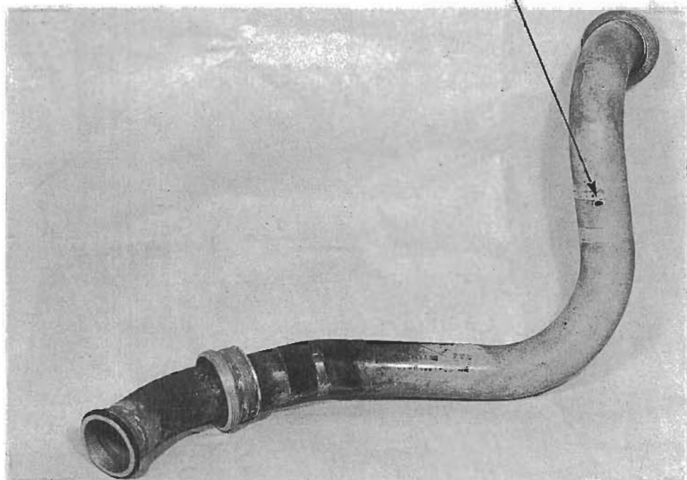
Damaged Portion of No. 2 Engine Fuel Feed Pipe (Hole)
