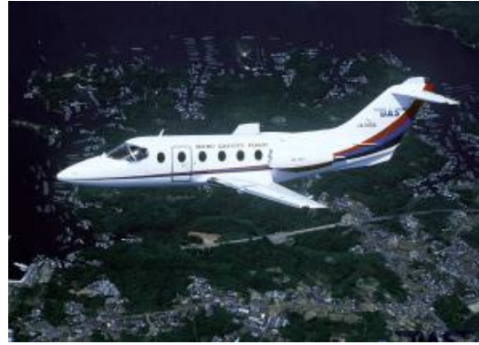
JA30DA (Mitsubishi MU-300) Over-all length 14.75 m Wing span 13.29 m Height 4.24 m
