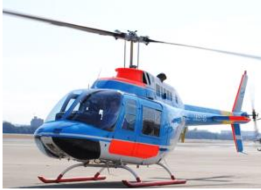
JA9745 (Bell 206B) Over-all length 11.92 m Width 2.07 m Height 3.26 m Main/tail rotor diameters 10.15 m/1.65 m
