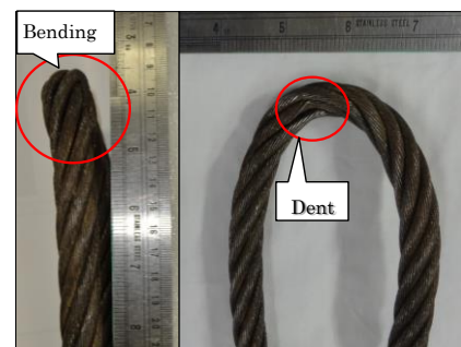
Photo 6: Condition of Improper Wire Hooking
