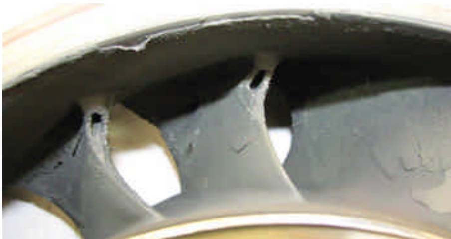
Heat erosion of inter-turbine vane airfoils
