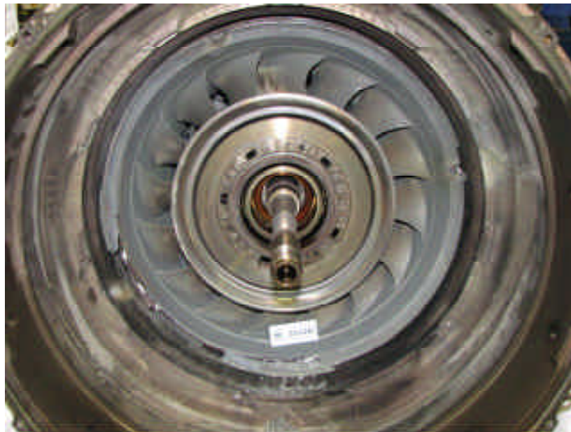
Inter-turbine vane (trailing edge side)
