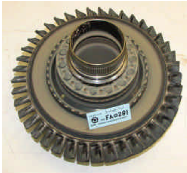
Photo 22 HPT disc – leading edge side
