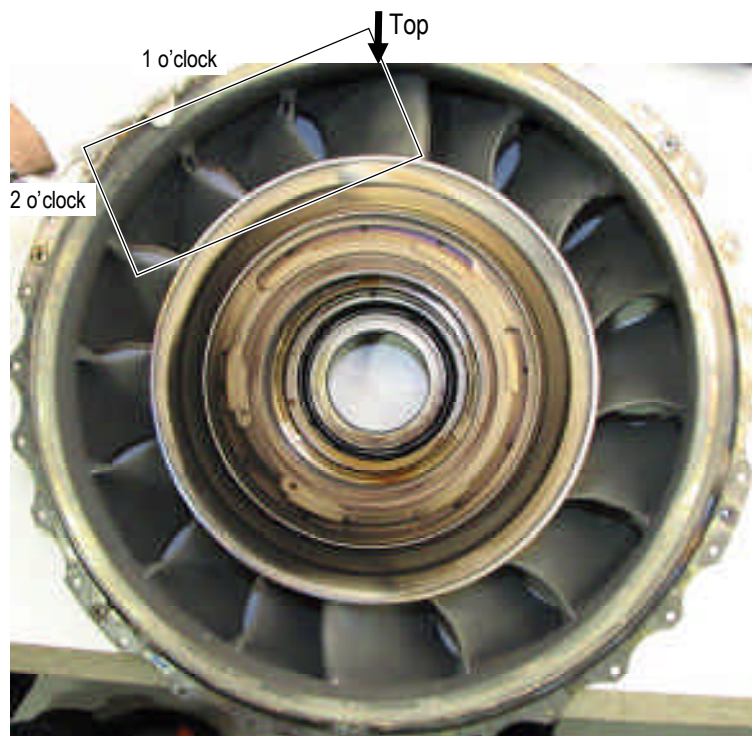
Photo 14 Inter-turbine vane – leading edge side
