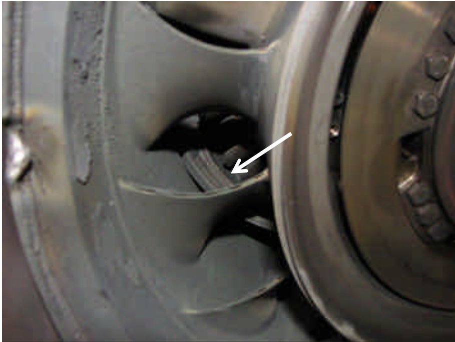
Inter-turbine vane (trailing edge side)
