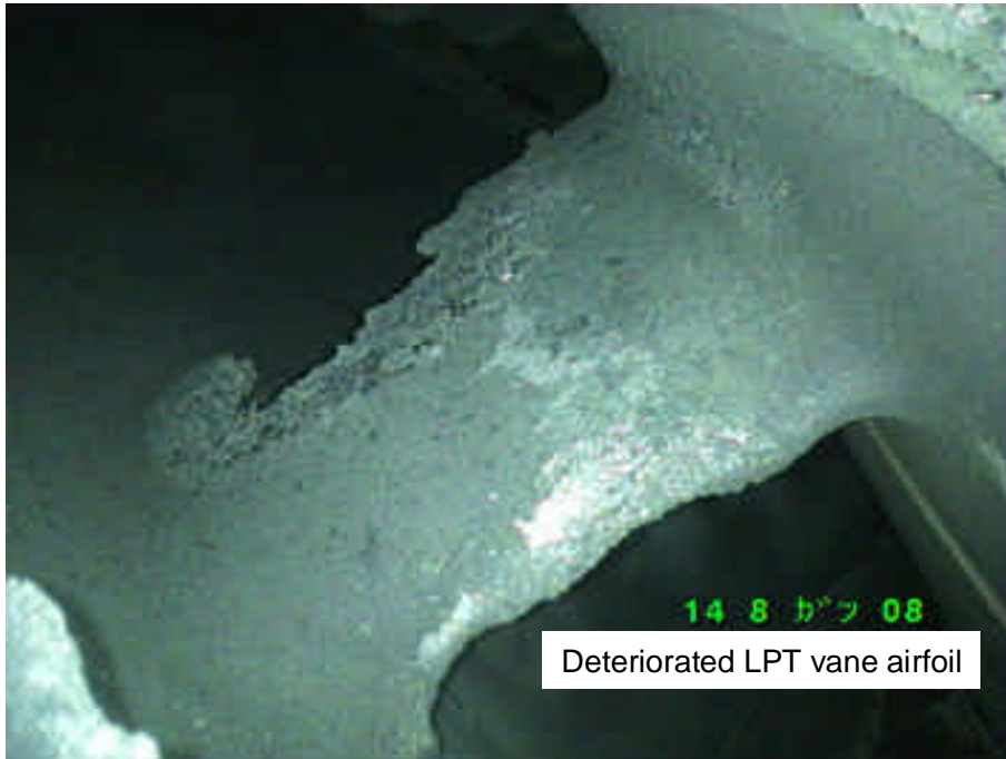
Photo 7 Deteriorated LPT vane airfoil (BSI view)
