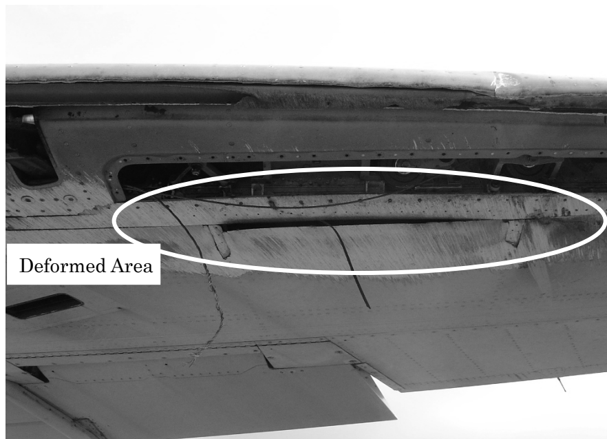
Photo 4 Deform of L/H Fwd Lower Spar
