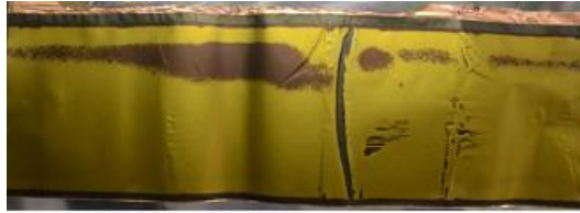
Fig. 2.13.2-1: Wrinkles of Anode Graphite during Narita Event Investigation
