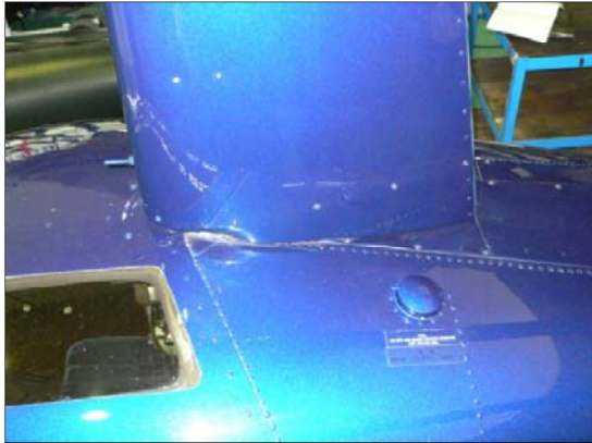
Deformity of the left lower part of the mast fairing
