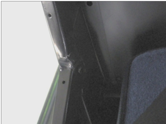
Corn buckle of the frame of the right side door
