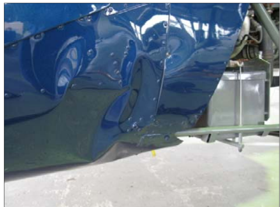
Corn buckle of the outer skin on left side of the fuselage
