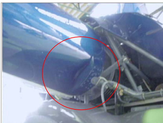
The tail corn buckled in the direction at five o'clock
