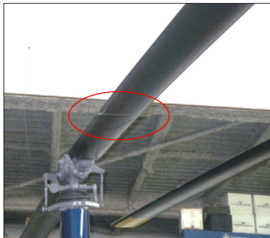
Wrinkle of the bottom side of one main rotor blade
