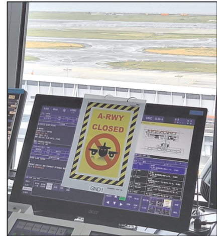
Figure 5: Example of How the Reminder is used (When a runway is closed)
