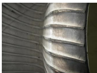
Photo 2.8.4-1 Inside of main landing gear tire inner pressure (165 psi).
