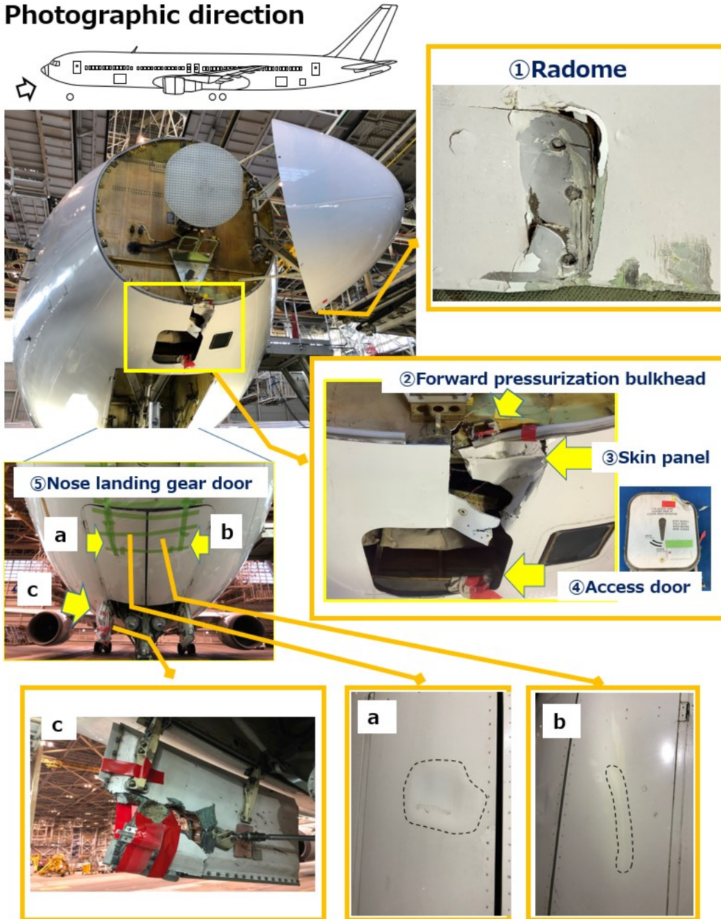
Attached Figure: Damage to the Aircraft
