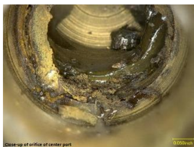
Photo 3: Examination of Fuel Selector Valve Photo 4: Substances adhered to the Valve outlet port
