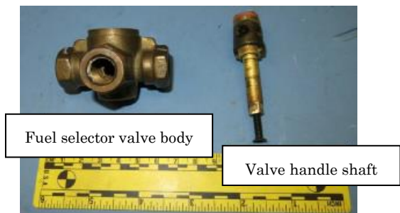
Photo 3: Examination of Fuel Selector Valve Photo 4: Substances adhered to the Valve outlet port
