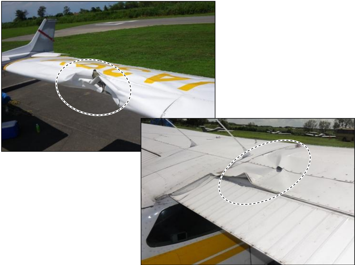
Photo 3 Damage to the Right Wing
