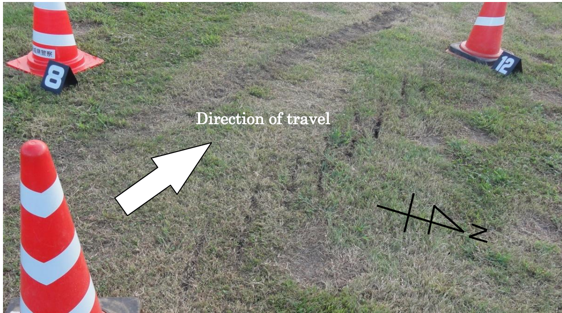
Photo 5 Slash Marks of the Propeller Blades on the Grass Area
