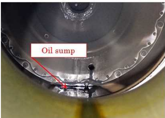
Inside of tailpipe of No.2 Engine
