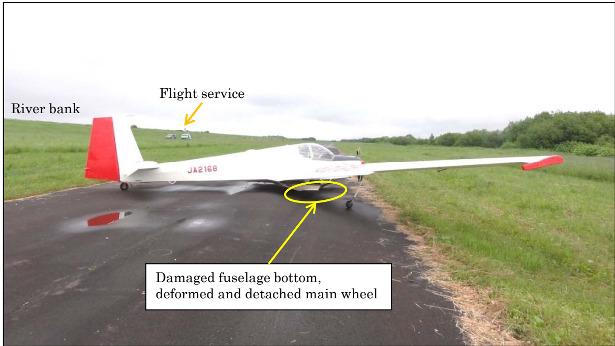
Deformed and detached main wheel
