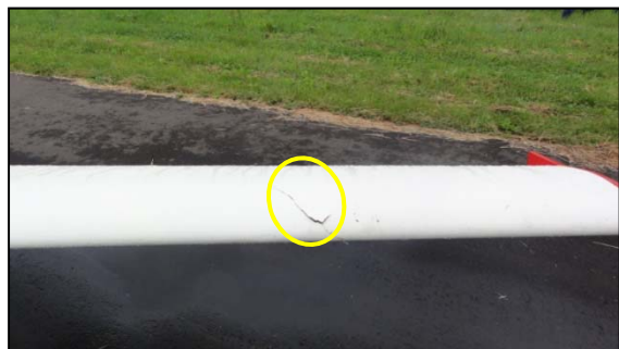
Cracked left wing
