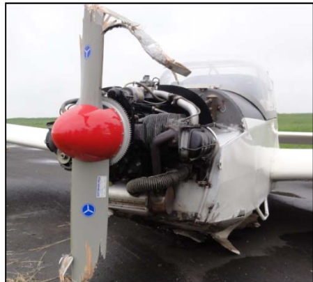
Broken propeller blades
