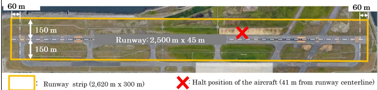
Figure 2 Runway strip of runway 10/28 at Niigata Airport (aerial photograph of Google Earth with some explanatory modifications added)
