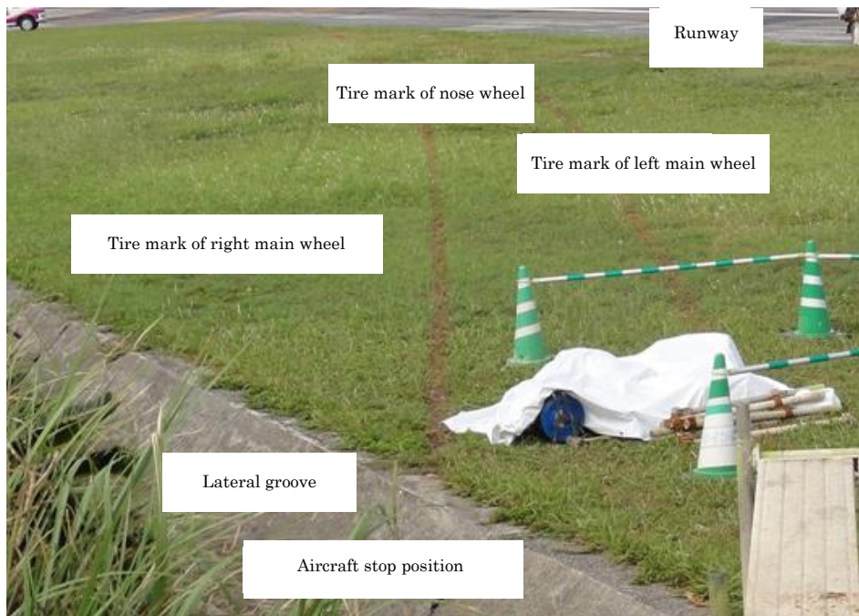
Photo D Tire marks just before the collision with the Perimeter Fence (See Annex Fig.1: Estimated Flight Route and Accident Site, Photo: Accident Aircraft)
