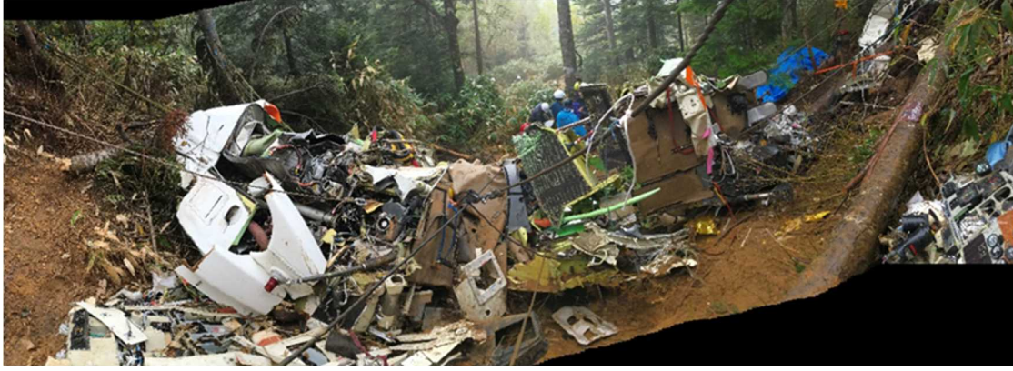
Figure 15: Damage from nose to aft fuselage
