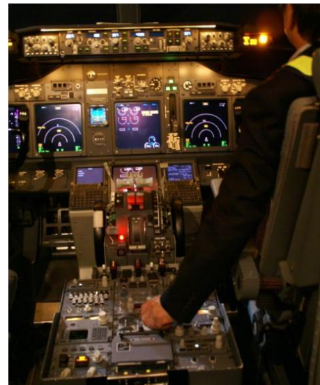
Operation of Rudder Trim SW
