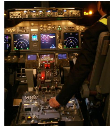
Rudder Trim SW operation (demonstration)
