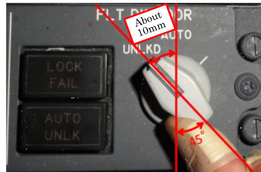
Shift amount of Door Lock Selector (737-700)
