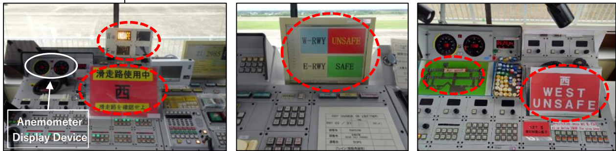
Figure 9: Reminders used at the airfield traffic control tower (from left, at the tower control position, at the Coordinator, and at the ground control position)
