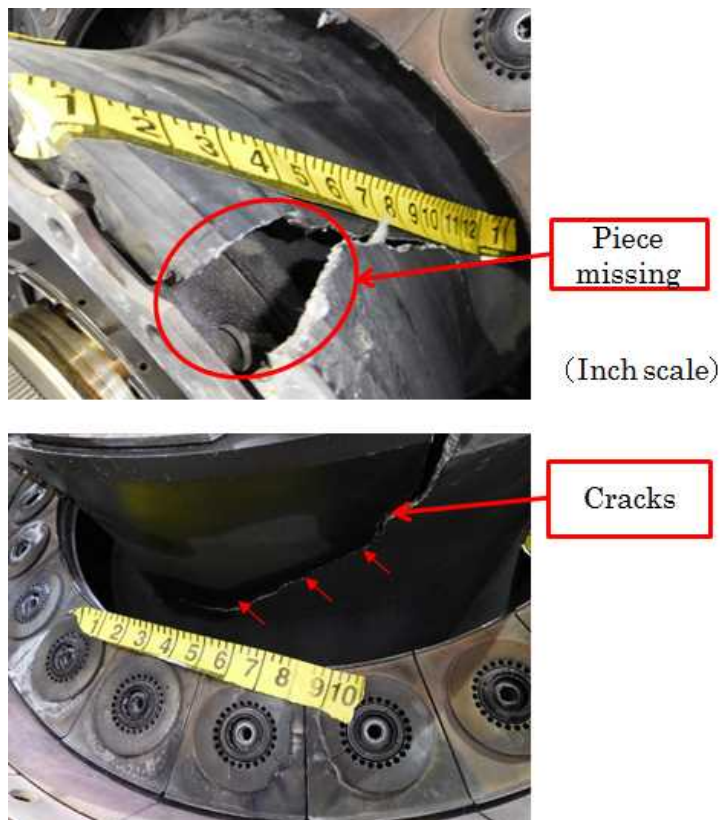
Photo #5. Inner diffuser case
