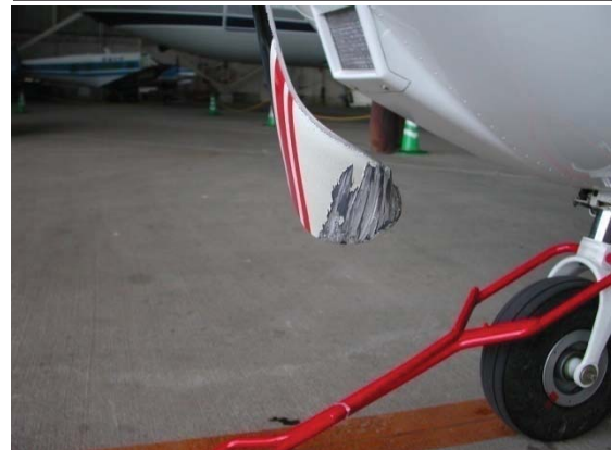
Damage of the propeller blades
