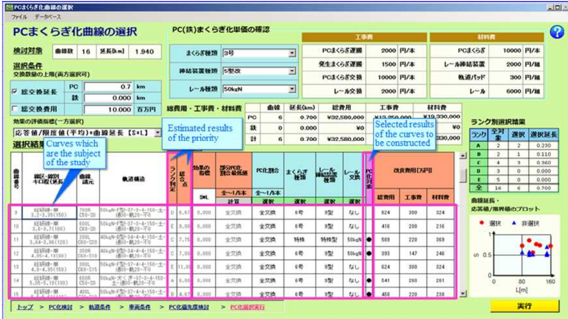
Display indicating the estimated and selected results of the priority and the target curves for the replacement to PC sleepers.
