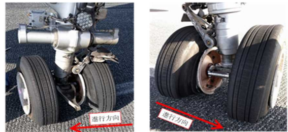
Damages to the nose landing gear of the Peach Aviation Limited's aircraft
