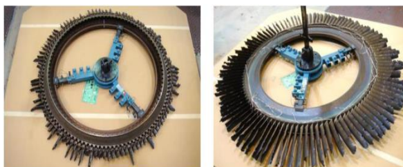
Damaged condition of LPT fifth stage disk and blades (left) and sixth stage disk and blades (right)
