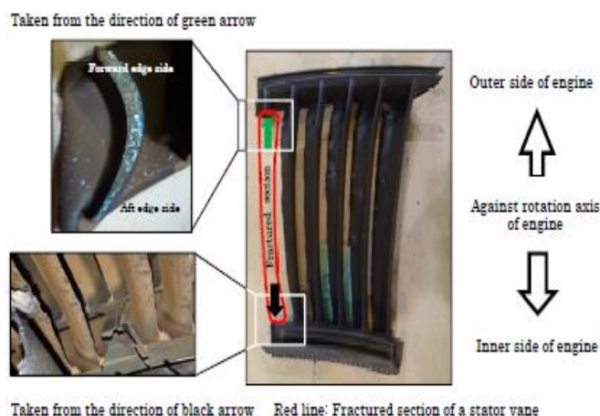
2LPT Missing vane in the fifth stage vane segment
