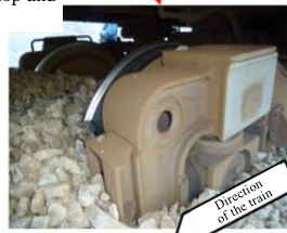
1st axle buried in piled gravel buffer stop (left side)
