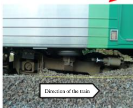
Front bogie buried in piled gravel buffer stop (right side)
